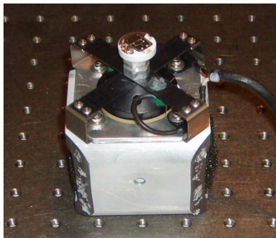
Figure 3.9: (a) A picture of the experimental setup used for testing the capacitive accelerometer at reduced pressure. (b) A picture of the shaker used to generate shock pulses inside the vacuum chamber.
